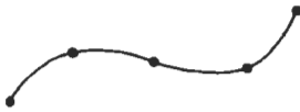
Figure 3-26 A spline curve formed with individual cubic polynomial sections between specified coordinate points.
