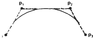
Figure 10-43 Quadratic, periodic B-spline fitted to four control points in the xy plane.
