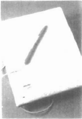
Figure 2-48 The NotePad desktop tablet with stylus. (Courtesy of CalComp Digitizer Division, a part of CalComp, Inc.)
