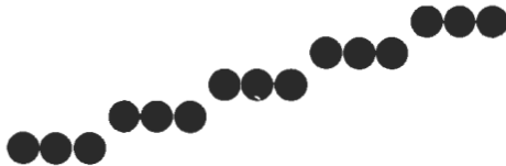
Figure 3-1 Stairstep effect (jaggies) produced when a line is generated as a series of pixel positions.
