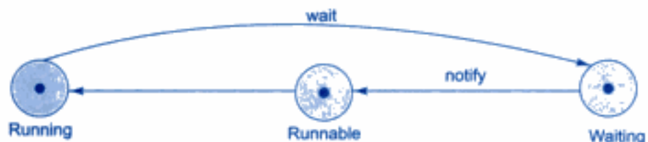
Fig. 12.8 Relinquishing control using wait() method
