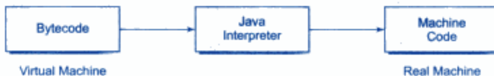
Fig. 3.7 Process of converting bytecode into machine code
