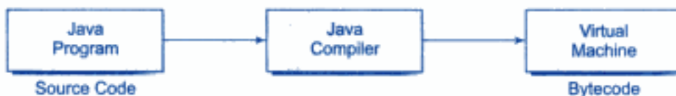
Fig. 3.6 Process of compilation
